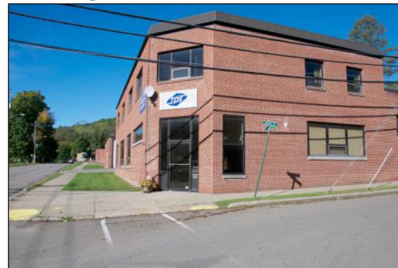
Do This: The TDS Telecom Building on Front Street is an example of an in-fill building, which complements adjacent buildings in terms of building alignment, massing, height, scale and form. This facility consists of two buildings with an alley that provides access to truck bays, while concealing these service area from Front Street. Street trees could have been planted along the front of the building to further tie this site into the downtown core.
