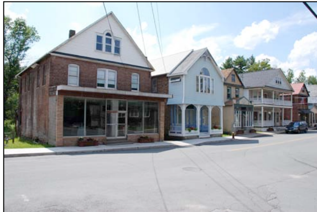
Above: Gable rooflines predominant Mountaindale's Main Street. A large percentage of its mixed-use buildings also have front porches. These design elements should be incorporated into the design of new infill buildings.
