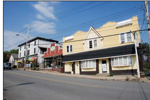
Above: View of Main Street Hurleyville that shows a number of historic structures with flat roofs. A parapet wall is used to conceal the roofline and add mass to the first three buildings. Unfortunately, the bay windows in the yellow building do not complement the buildings original design.
