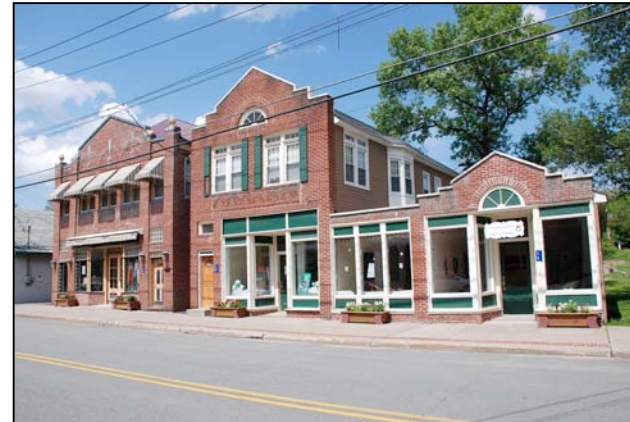
Above: View of Main Street Mountaindale looking north. Again, gable rooflines predominant Mountaindale's Main Street. Notice the one-story structure incorporates a parapet to add mass and scale to the structure. Building size, setbacks, and rooflines help to define the character of this hamlet center.
