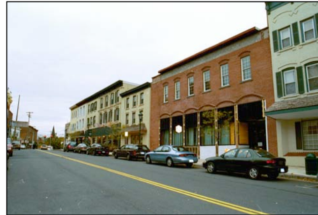
Above: Core of Historic Downtown Walden showing predominant building heights, setbacks, and roofline. The infill building front right incorporates a horizontal roof. This photo shows façade renovation in progress.
