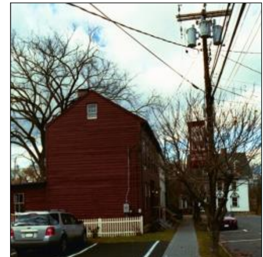
Illustration: Street tree placement should take into consideration the presence of utilities underneath or electric wires overhead. Trees should be selected such that mature tree height is less than the height of any wires, or trees should be pruned below wires. Source: Planning & Urban Design Standards.
